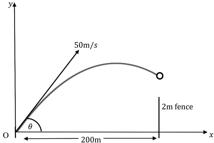
A ball is hit at 50 m/s. The fence, 200 metres away, is 2 metres high. You may neglect air resistance and acceleration due to gravity can be taken as  $10 \text{ m/s}^2$ . You may assume the following equations of motion:
